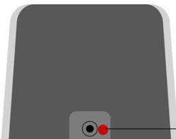
Star-shaped screw hole for fixing a body to a metal bracket
